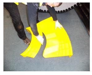
Separate outer shield from inner shield whilst on floor.
