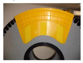
Place outer shield onto top surface of coil. (12 o'clock position)
